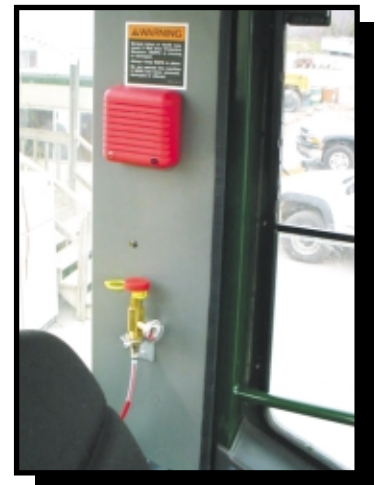
Image 4 - Manual Release and Audible Alarm mounted in the cab
