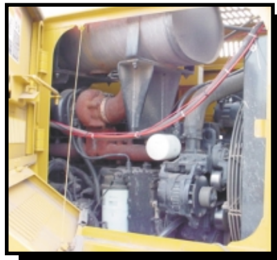
Images 2 & 3 - Firetrace Detection Tubing mounted in the engine compartment
