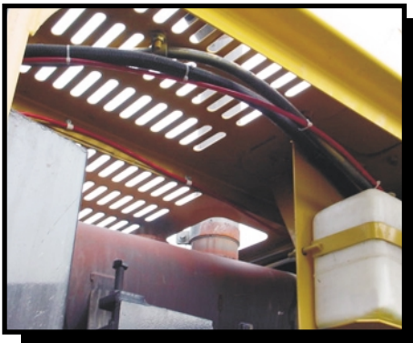
Images 2 & 3 - Firetrace Detection Tubing mounted in the engine compartment
