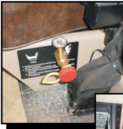
Manual Release and Audible Alarm are located in the cab.
