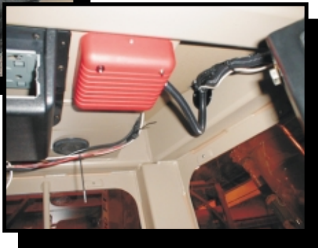
Manual Release and Audible Alarm are located in the cab.
