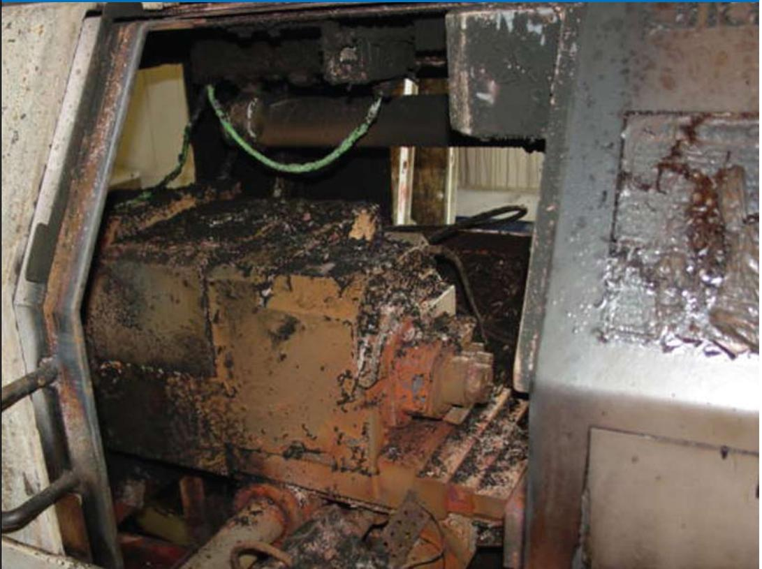
The damage caused by a machine fire can inflict substantial losses on a machine shop. Sometimes the entire facility is a total loss. Left undetected, a machine fire can quickly spread to neighboring equipment or to the building's structure. Even when the building sprinkler system activates, the machine, and often much more, may be destroyed.
