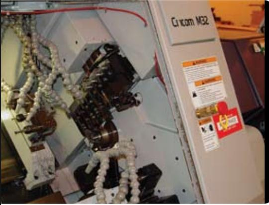
Supplementary fire suppression systems are designed to extinguish a fire at its source within the machine. The red pressurized Firetrace tubing running across the top of this turning center's enclosure is part of the fire suppression system installed on the machine.
