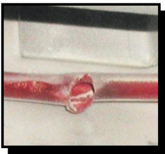
**Image 3** Actual burst on detection tubing
