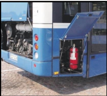
Image 3 - Firetrace system installation.
