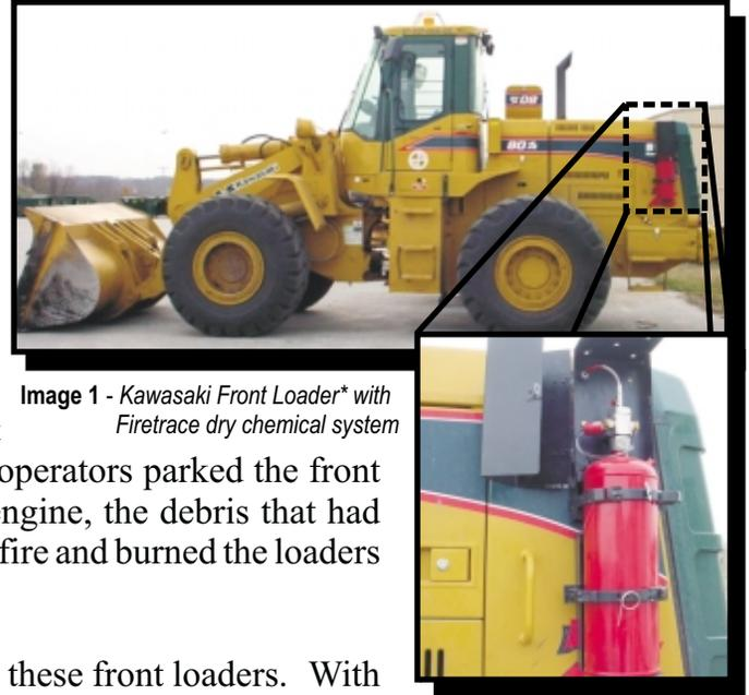
Image 1 - Kawasaki Front Loader\* with Firetrace dry chemical system
