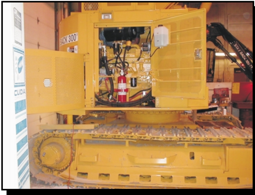
Firetrace Indirect Low Pressure (ILP) System protects the engine compartment from fire.
