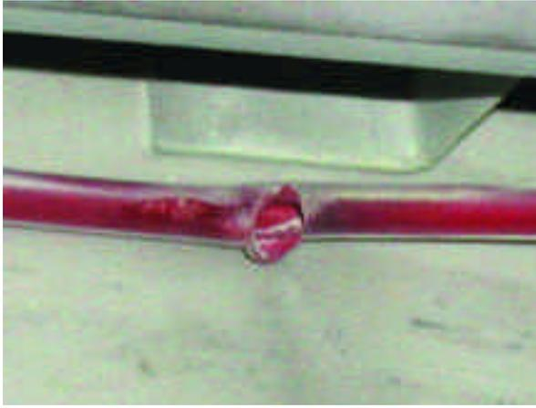
**Figure 1** An actual tubing burst from a fume cabinet fire.
